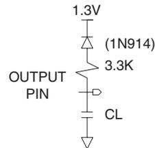
Note:  $CL = 100 \text{ pF}$  including jig capacitance.
